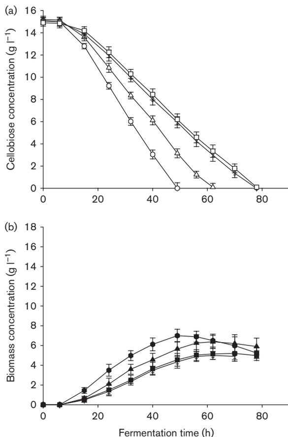
**Fig. 7.** Time profiles of residual cellobiose concentration (a) and growth (b) in batch fermentations of the monocopy *lacpB* retransformant (up-pointed triangles), the *lacpA* deletant (hexagons), the *lacpB* deletant (squares) and the *lacpA/lacpB* double permease deleted (female symbols) *A. nidulans* strains. The monocopy retransformant essentially behaves like wild-type control strain R21. Media were inoculated with conidiospores.
